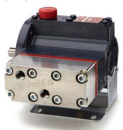
Following extensive on-site testing, Hydra-Cell Go4 pumps have now been uprated to 200 Bar when operated at a reduced speed and with a commensurate reduction on flow rate. The pumps are now rated at 5.65 litres per minute at 200 bar pressure and 11.3 litres per minute at 170 bar.
